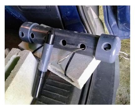
Figure 2: Dissolved Oxygen Logger Housing and Cinder Block Anchor
